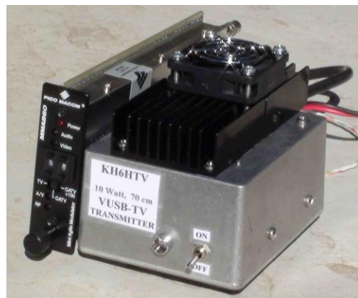
Fig. 7 KH6HTV, 10 W, 70 cm, synthesized, VUSB-TV transmitter
