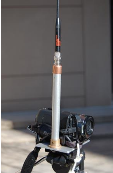
Fig. 5 The Sony hi-def. camcorder and 70 cm, whip antenna, both mounted on a tripod.
